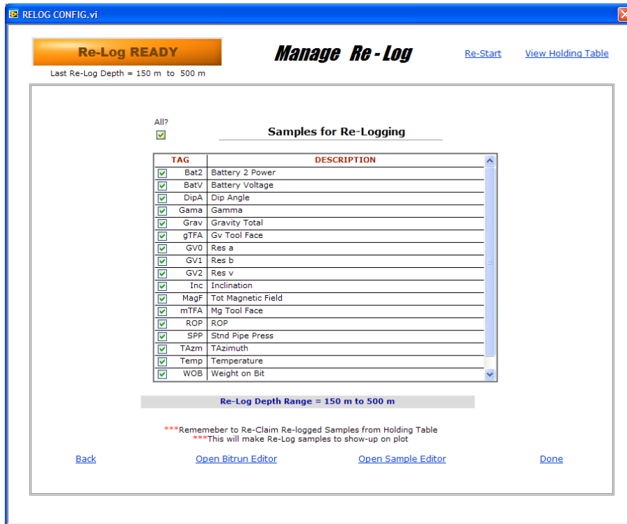
Figure 122. Choose samples that you want to Re-Log. If not sure, just leave all samples checked. However, usually only Gamma is clicked. ROP is meaningless when re-logging. The orange indicator means that Re-Log is now ready to happen (armed). That Indicator will turn Green if the Bit Run is within the depth of the re-logging range.
