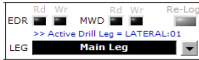
Figure 89. The note in blue text reminds the user that the well bore selected is not the active one which is collecting new drilling data. You can select a well bore different than the active one to review data or to plot data for that well bore.
